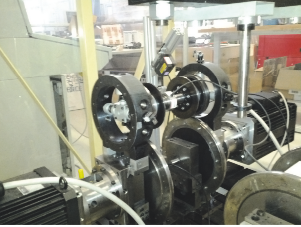
FIGURE 1: Roller-rig with a single suspended wheelset.
