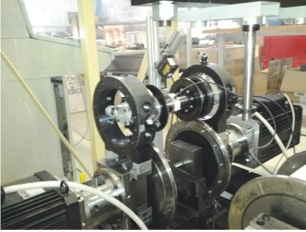
FIGURE 1: Roller-rig with a single suspended wheelset.
