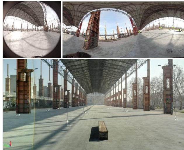
Figure 10. An example of spherical image from GoPro Fusion 360° (one fish-eye hemisphere), and planar view; (bottom) adjusted camera station points from V10 Trimble rover.
