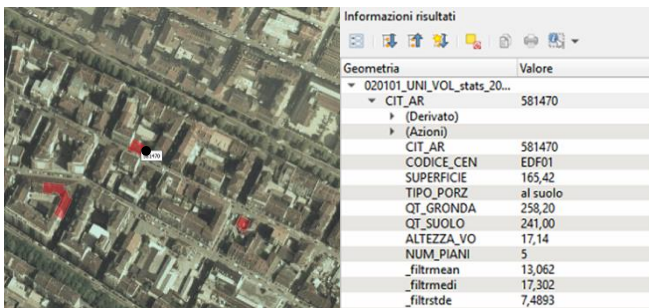
Figure 6. Correspondence check between DSMD statistical values and digital mapping of Torino, red. Volume data analysis on a sample with attribute about “Volume height”
