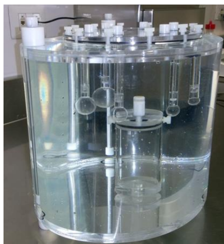
Figure 1 NEMA PET-TC phantom
