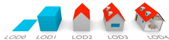
Figure 1. Level of Detail for CityGML standard.
