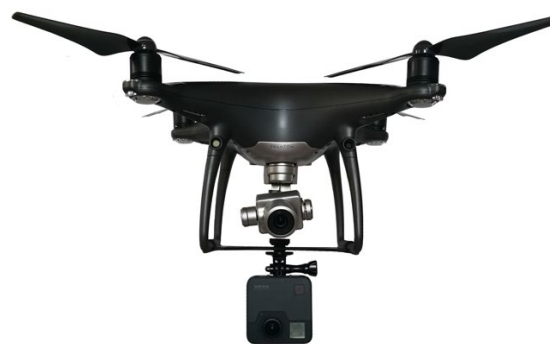
Figure 1. The UAVs/360° camera set up adopted in this research to perform a double sensor acquisition.
