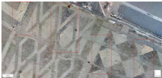
Figure 13. Details of the radiometric and resolution discontinuity in orthophoto generated using images from both sensors.
