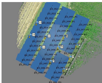
Figure 5. Project A, orientation of oblique images and extracted tie-points (sparse cloud).
