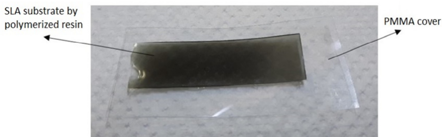
Fig. 2. Sample composed by SLA polymerized resin and PMMA cover.
