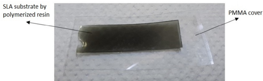
Fig. 2. Sample composed by SLA polymerized resin and PMMA cover.
