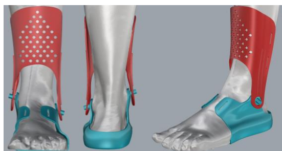
Fig. 7. Views of a HAFO prototype 3D model obtained on the scan of the subject's limb.
