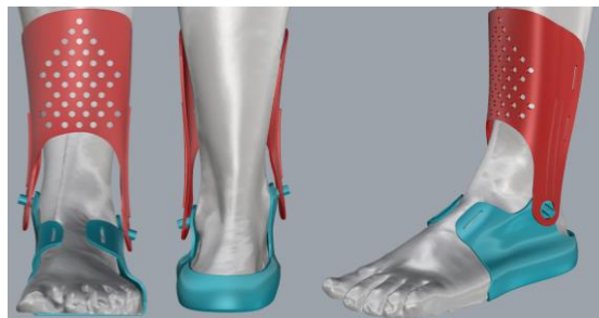
Fig. 7. Views of a HAFO prototype 3D model obtained on the scan of the subject's limb.
