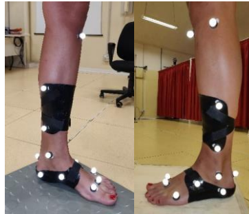
Fig. 6. Example of partial shells for the in-vivo analysis of ankle joint kinematics.
