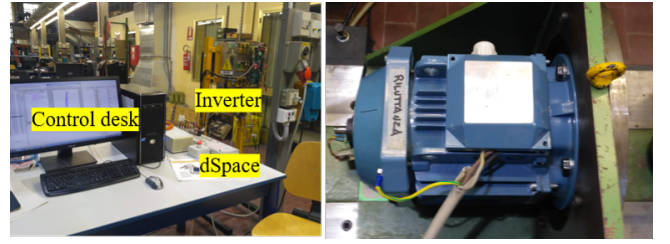
Fig. 4. Experimental Setup of 1.1 kW SyR motor under test.
