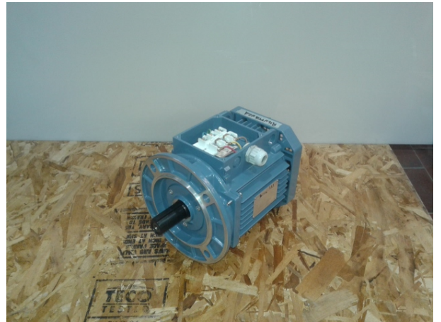
Fig. 6. SyR motor under test (1.1 kW).
