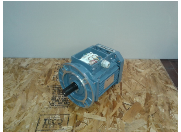
Fig. 6. SyR motor under test (1.1 kW).
