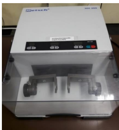
Figure 2.3 Picture of the Retsch MM 400 bead milling device.
