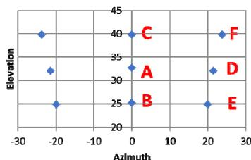
Fig. 6. Feed positions in the vertical plane and corresponding beam peak directions.
