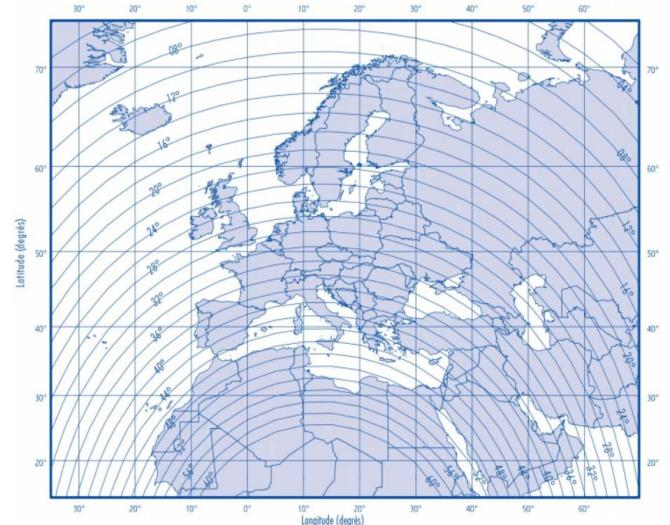
Fig. 1. Elevation angles for Eutelsat 13° position.
