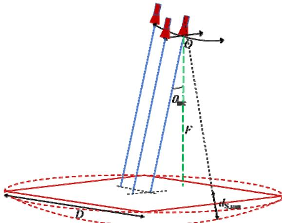
Fig. 3. Geometry of the reflectarray with the spherical surface whose behavior is emulated.
