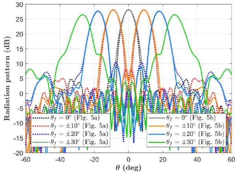
**Figure 21 - Radiation patterns in the E-plane relative to the dielectric TA, illuminated by a horn that translates parallel to the TA as in Fig. 8b (dotted line) and compared with the case in which the horn rotates along a circular arc as in Fig. 5a (solid line).**
