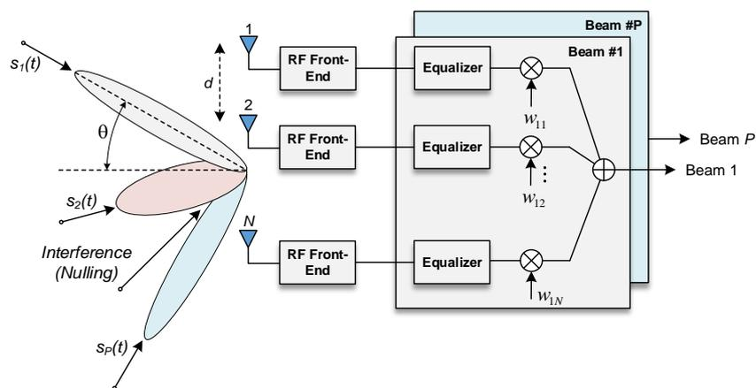
**Figure 12 - Multi-beam phased array architecture.**
