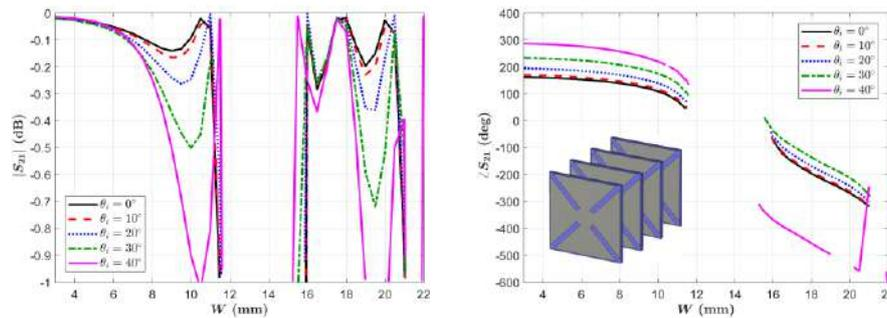
**Figure 16 - Variation of the amplitude (left) and phase (right) of  $S_{21}$  versus  $W$  for several angle of incidence. Inset: unit cell.**
