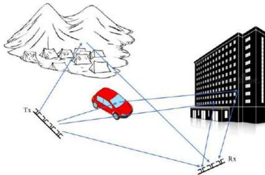
**Figure 11 - Sketch of an outdoor environment, where several transmitting and receiving devices are present. The wireless connection is carried on taking advantage from the multiple reflections as in a MIMO system.**
