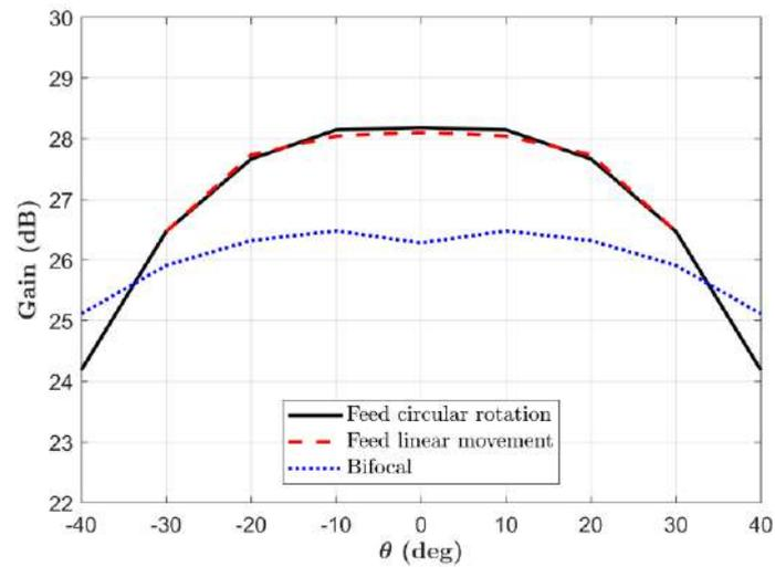
**Figure 24 - Variation of the gain versus scanning angles. Comparison among the conventional TA, illuminated with a feed that moves along a circular arc (solid line) or linearly (dashed line), and the bifocal TA (dotted line).**
