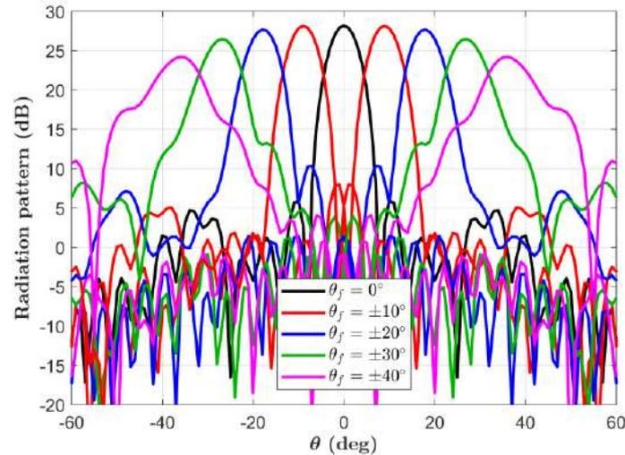
**Figure 20 - Radiation patterns in the E-plane relative to the dielectric TA, illuminated by a horn that rotates along an arc centered in the center of the transmitarray aperture (configuration in Fig. 8a).**
