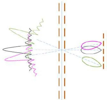
**Figure 15 - Working principle of a multibeam TA: each element in the feed array radiates a beam in a different direction, that impinges on the transmitarray with a different angle of incidence that generate a beam in the consequent direction**
