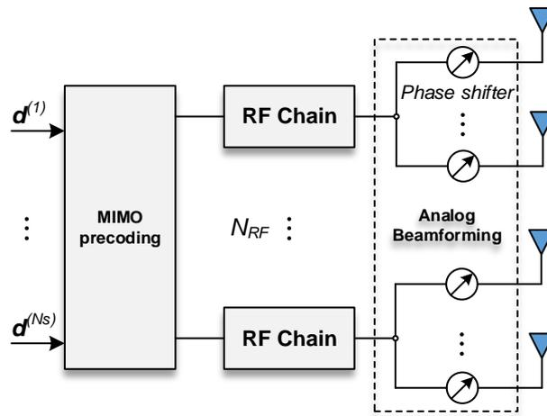
**Figure 14 - Hybrid beamforming structure for the mm-wave transmitter.**
