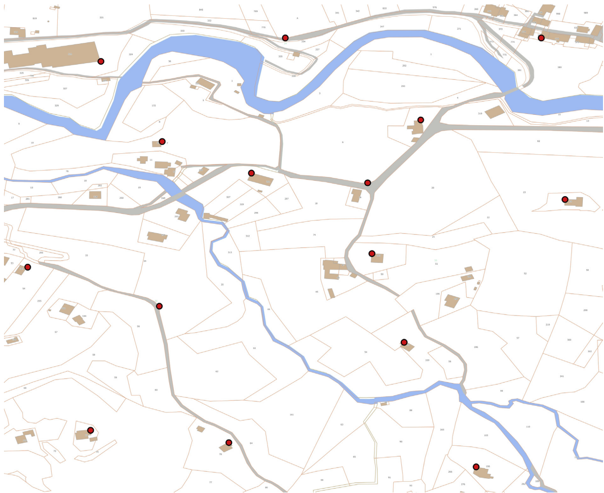
Fig. 3. The 15 points measured with the NRTK technique considering GNSS mass-market receiver and antenna.
