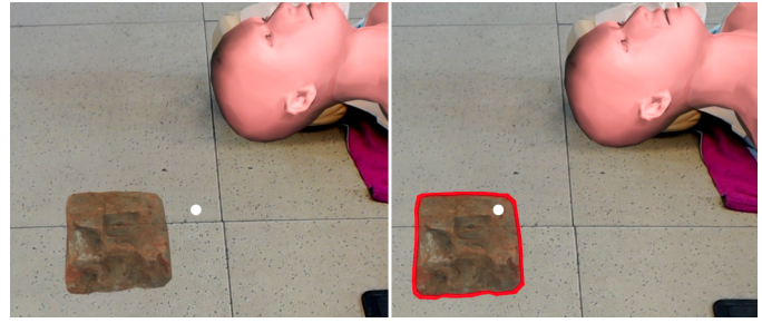
Fig. 5. Highlighting of a gaze-selected, or -targeted, object (the white dot is the gaze cursor).
