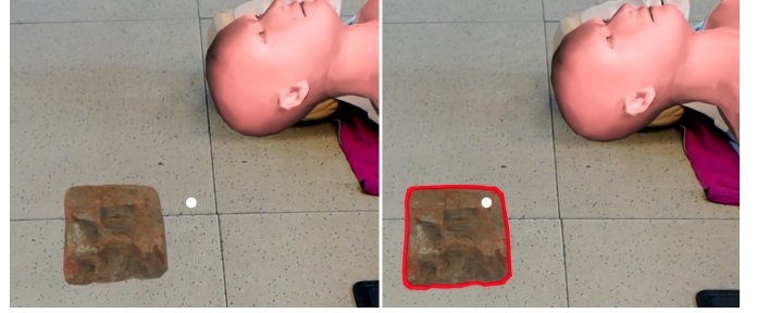
Fig. 5. Highlighting of a gaze-selected, or -targeted, object (the white dot is the gaze cursor).
