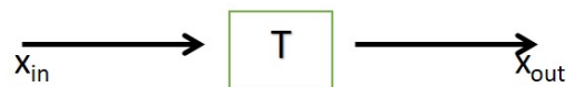
Figure B.1: Transfer Function with x_{in}(s) as input x_{out}(s) as output. T is considered as Transfer function.
