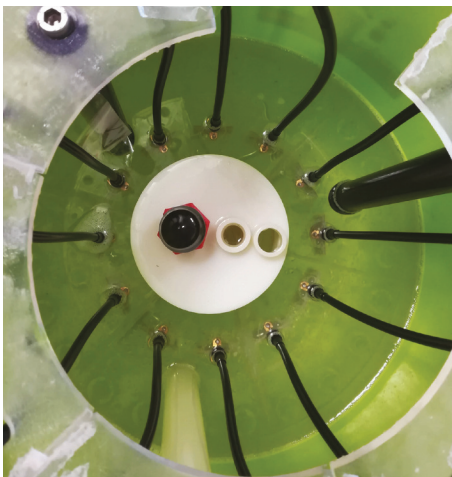
FIGURE 2: Microwave imaging system: tank filled with the coupling liquid with phantom and RX/TX antennas inside.
