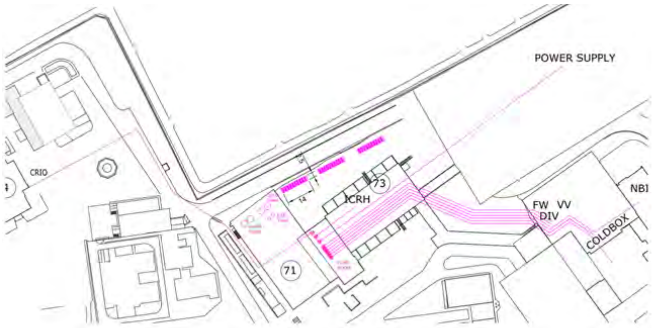
Figure V.7: Layout of the water-cooling system secondary loop.
