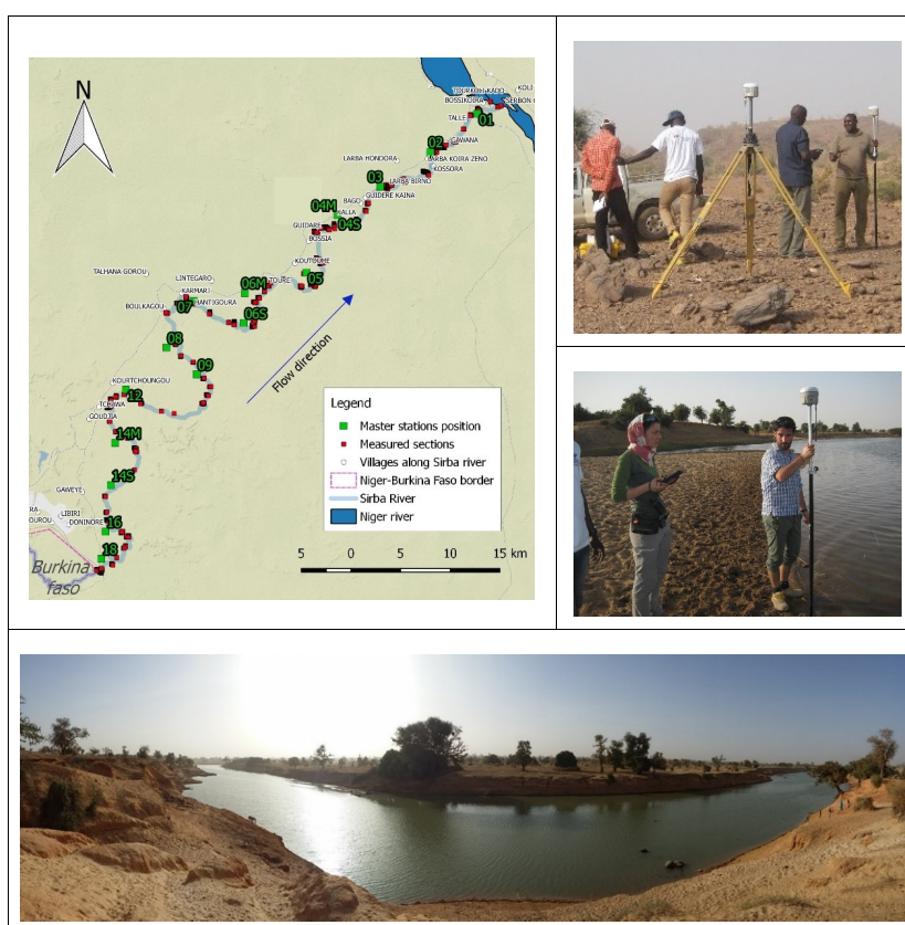
Figure 3. Above left: area of the topographical surveys: the green squares indicate the 18 stations along the river, while the red ones the sections along the river. Above right: the GNSS devices STONEX S10. Middle right: the topographical survey conducted on the field. Below: Panoramic view of the Sirba River near the village of Larba Birno.
