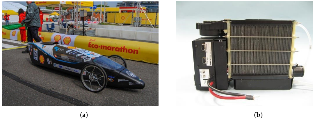
Figure 6. (a) The vehicle IDRA and its (b) Fuel Cell.
