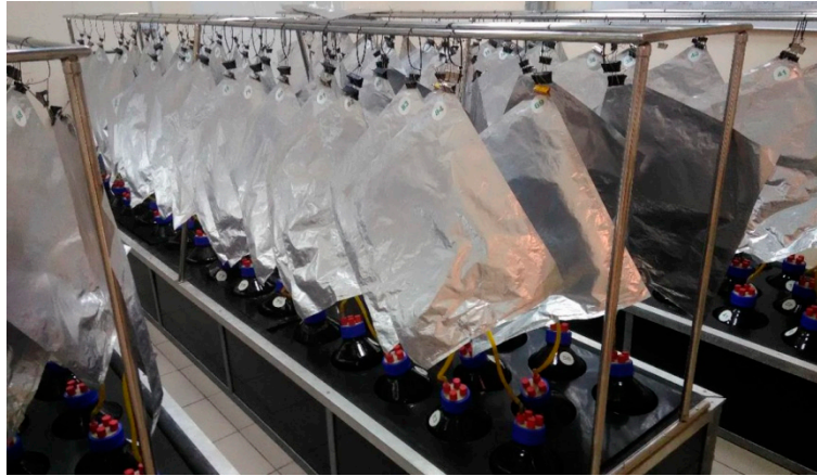
Figure 5. Mini-fermenters in laboratory.
