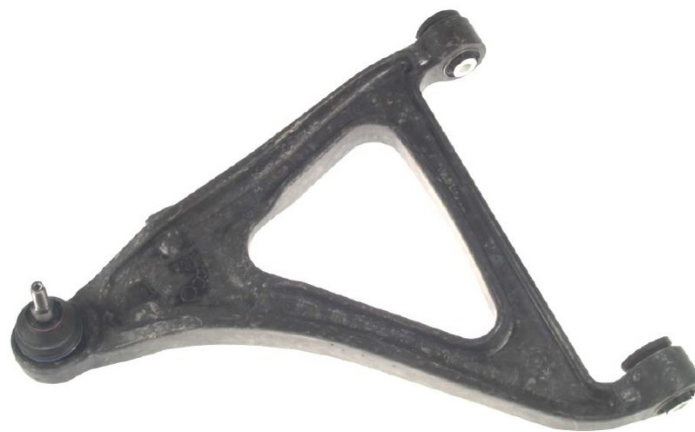
Figure 1.25 - Lamborghini LCA with thinned flange to increase stiffness
