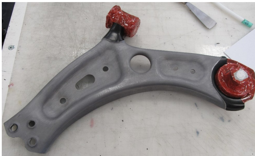
Figure 6.30 – Surface finishing before lamination
