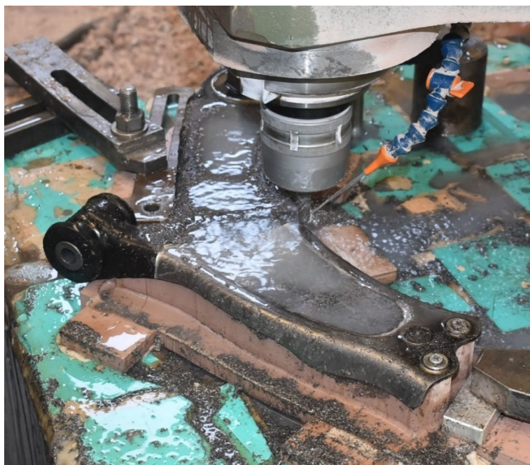
Figure 6.28 - Milling operation on LCA
