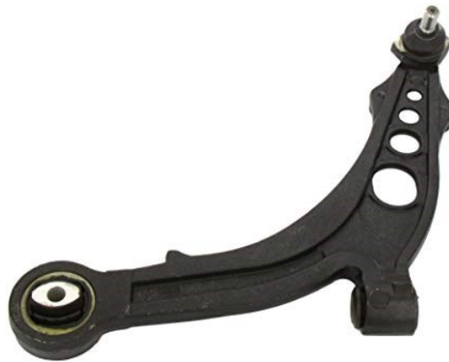
Figure 1.13 - The banana-like shape of a lower control arm
