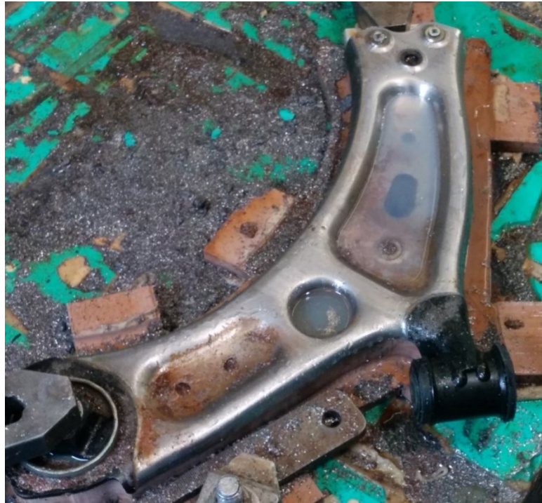
Figure 6.29 – LCA with reduced thickness metal part
