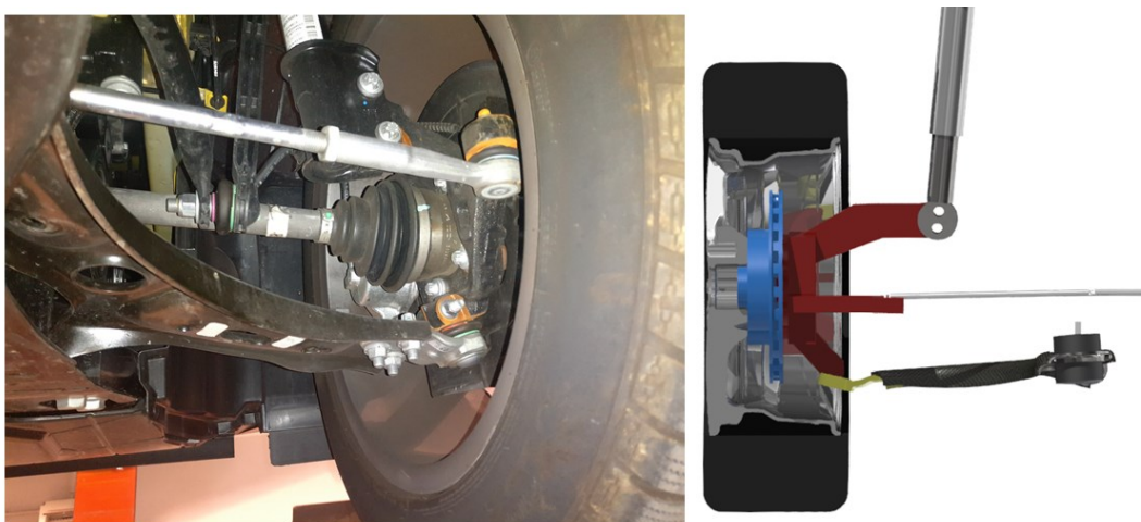
Figure 3.9 – Wheel assembly (left) and its simplified CAD model (right)
