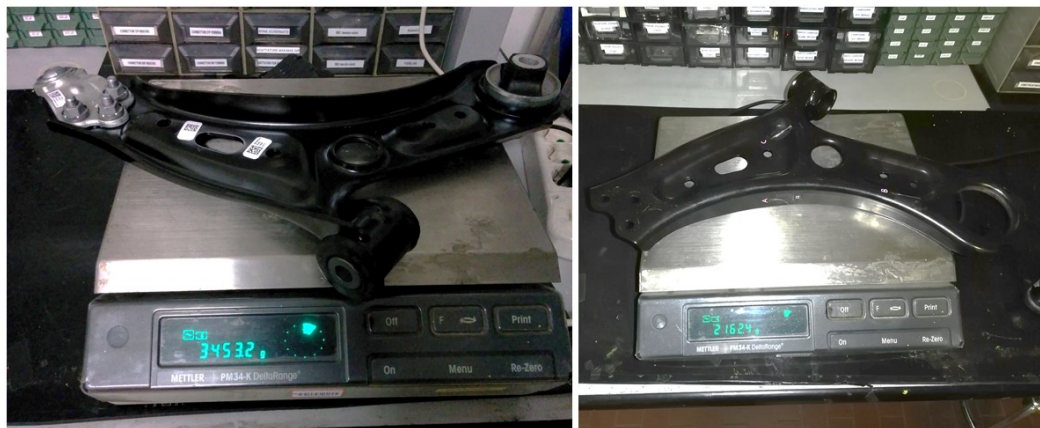
Figure 2.5 – LCA total mass (left) and without bushings and lower ball joint (right)
