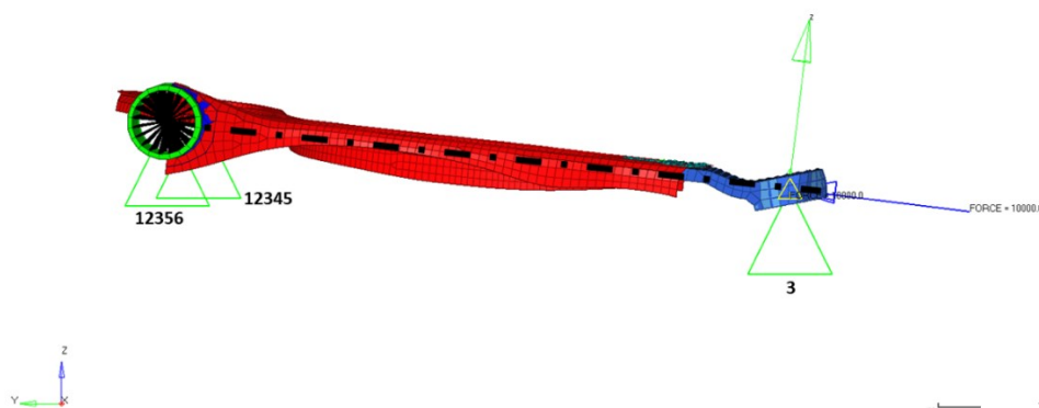
Figure 2.35 – LBJ reference system (green) oriented as in MBD model
