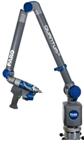
Figure 2.23 - Anthropomorphic laser arm
