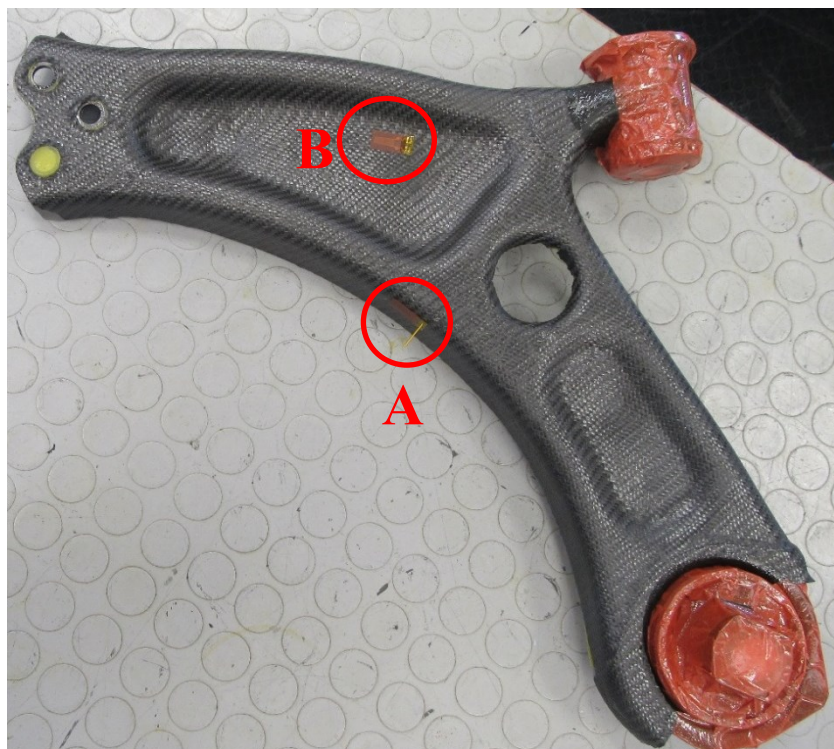
Figure 6.32 – First ply of GG245T with interlaminar strain gauges
