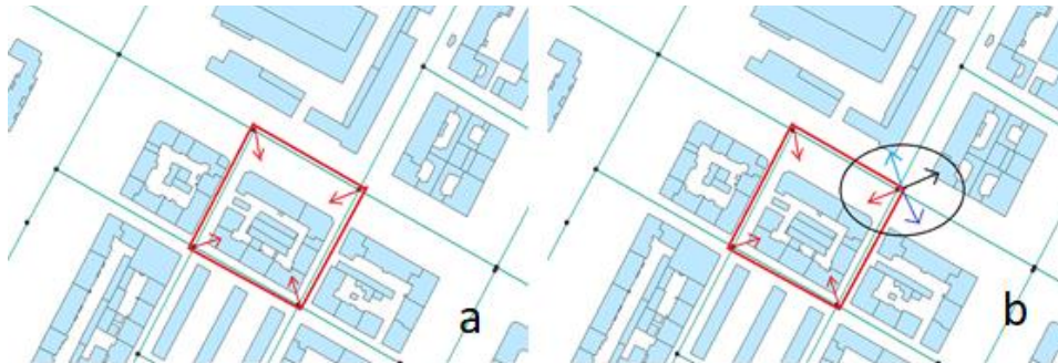
Figure 5.4 (a) Water demand q_{j,w} within a mesh element w , (b) Water demand at a node i .
