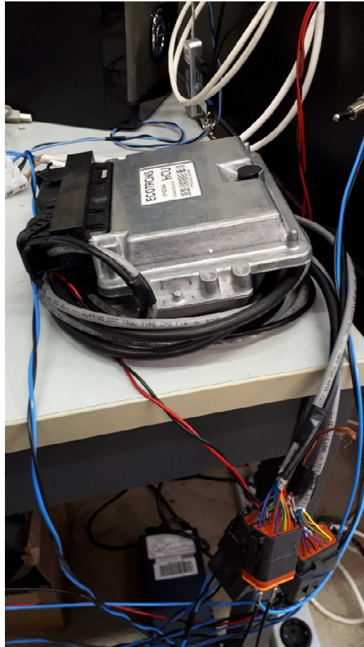
Figure 5.12 Hybrid Control Unit
