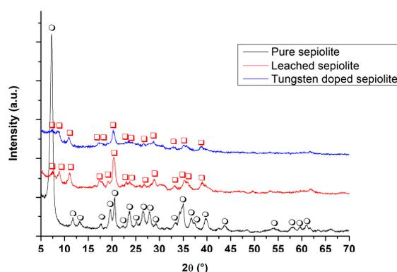
**Figure 1.** XRD pattern of pristine sepiolite, leached sepiolite, and heat-treated anhydrous sepiolite (○: sepiolite (JCPDS card n°13-595), □: anhydrous sepiolite [18]). Reprinted with permission from [20].
