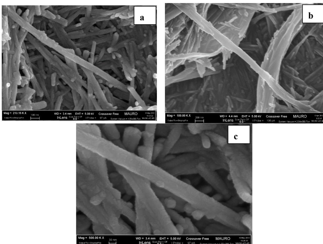
**Figure 2.** FE-SEM micrographs of: pure sepiolite (a); sepiolite thermally treated at  $550^\circ\text{C}$  for 1 h (b); tungsten-modified sepiolite after firing at  $550^\circ\text{C}$  for 1 h (c).
