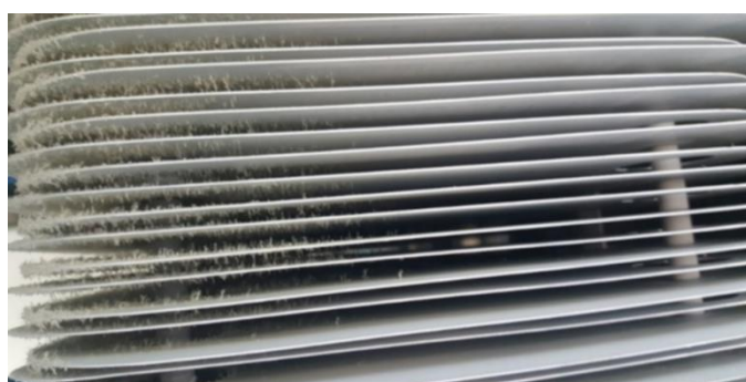
Figure 11. Top view of collection plates with progressive build-up of particles (fumes enter from left side)
