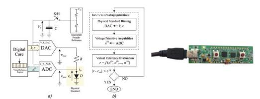
"virtual voltage reference" [2-3], where a process, supply and temperature independent voltage is obtained algorithmically starting from a possibly inaccurate pseudo-reference (see Fig.2) has been demonstrated on the basis of theory and of proof-of-concept prototypes. The same concepts are still being refined and investigated with promising results in terms of power consumption at very low supply voltage and are well suited to Internet of Things (IoT) applications.
