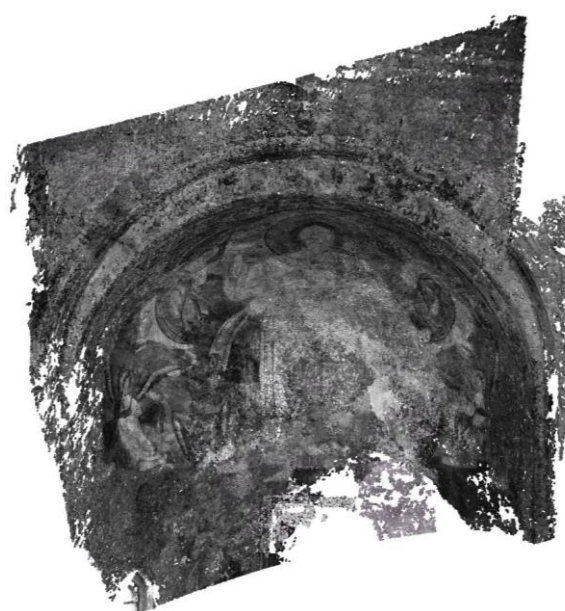
Figure 4. Dense cloud obtained from processed historical images.
