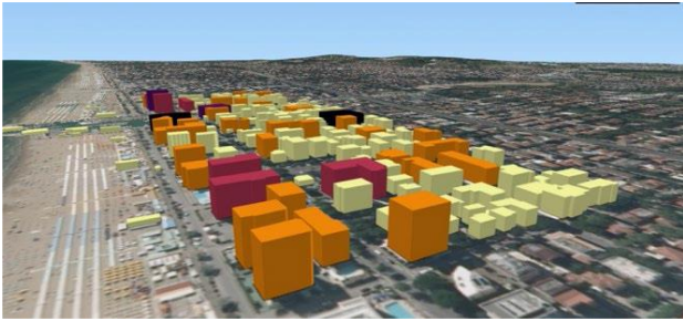
Figure 2. 3D City Model graphical representation with LoD1 buildings classified according to their new volume attribute.
