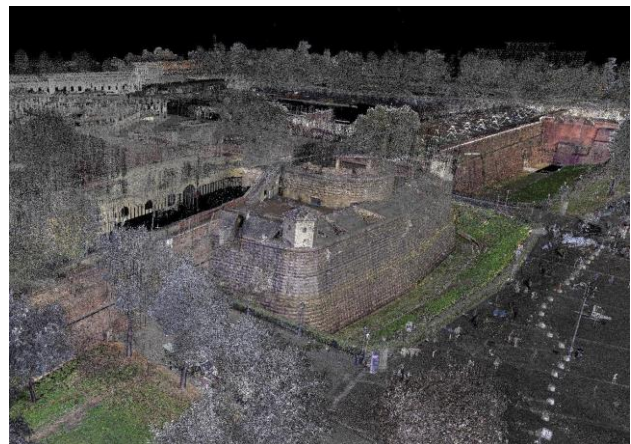
Figure 11. Point cloud generated by different sensors (Tucci et al., 2017)
