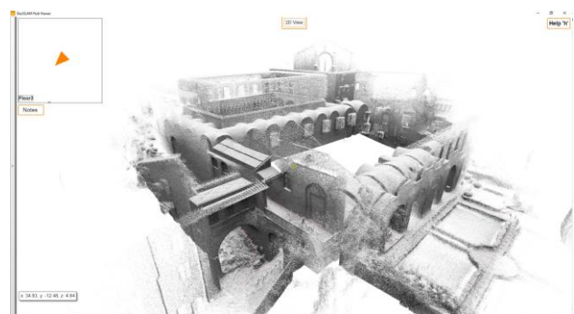
Figure 6. 3D visualisation and navigation through the point cloud within the Geoslam software.
