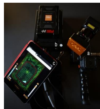
Figure 4. The ZEB-Revo RT system: (a) the handheld device mounting the rotating laser head in the upper part and below the Zeb Cam, (b) the data logger, (c) the tablet connected through Fi-Wi.
