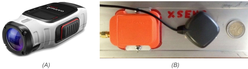
Figure 3.2. (A) Action cam Garmin VIRB® Elite; and (B) Xsens Mti-G IMU sensor with GPS antenna
