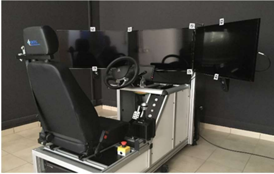
Figure 3.1. Current layout of the fixed-base driving simulator in the Road Safety and Driving Simulation Laboratory at the Politecnico di Torino
