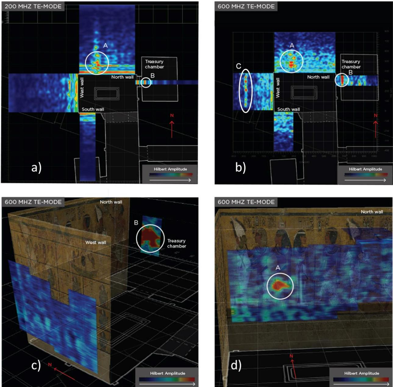
**Figure 5:** IF and LF processed data: top view of representative horizontal cross sections for a) LF processed data and b) IF processed data, vertical cuts at 0.6 m depth from the IF GPR volume (TE-mode) behind the west c) and north wall d) are also reported. Evidence of: A wall repair anomaly, B wall separating the Burial Chamber from the Treasury Chamber and C deep linear reflection event are reported in all the panels.
