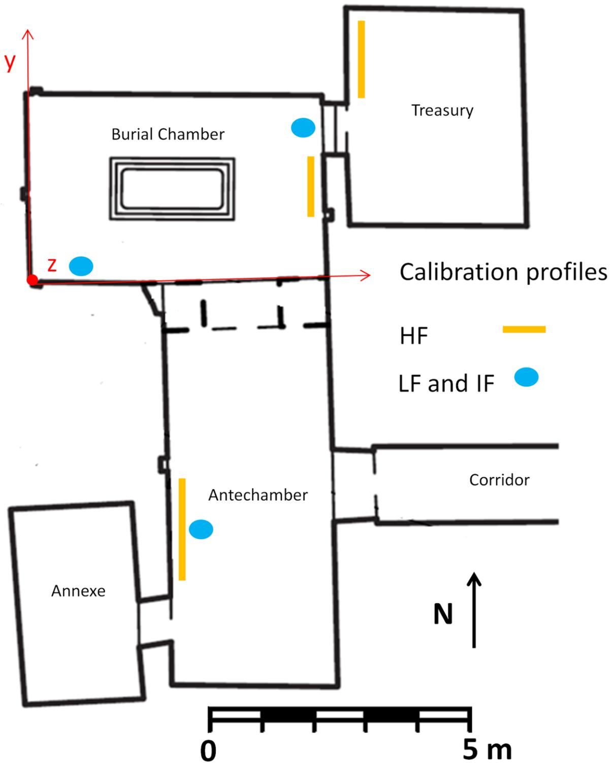
**Figure 1:** plan view of the KV62 with indication of the reference system used for survey positioning and the location of the calibration profiles: yellow lines are the HF scans profiles, cyan dots are the planar projection of the vertical LF and IF profiles (modified from Weeks, 2003).
