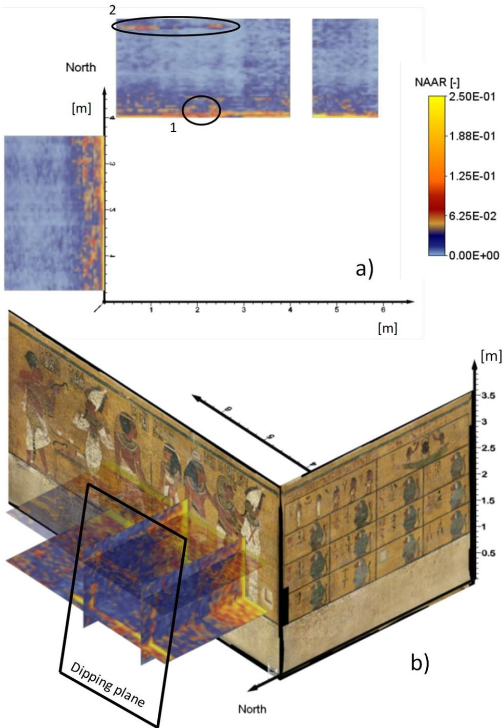
**Figure 4:** HF-TM mode processed data: a) Top view of the sections at 1 m from the floor, with evidence of: 1) high amplitude shallow events related to the wall repair and 2) a 2 m deep linear reflection event; b) 3D view of some significant sections: behind the North wall, a clear fracture plane emerges from the combination of vertical and horizontal sections.
