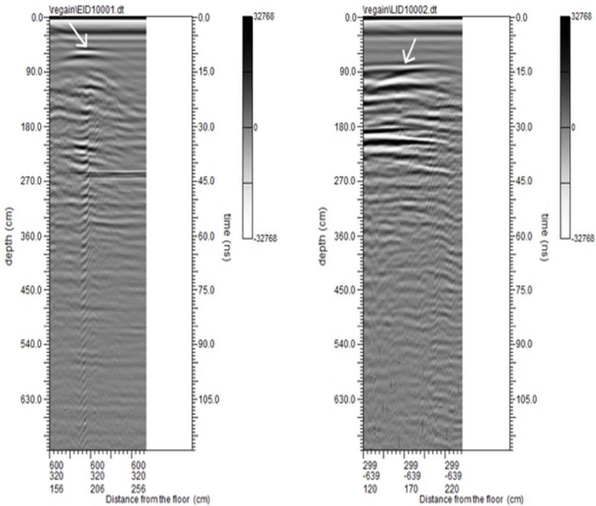
**Figure 6S:** LF calibration radargrams, at processing step 03, acquired along the East Wall of the Burial Chamber toward the Treasury(left) and along the West Wall of the Antechamber toward the Annexe (right),for exact location see Figure 1 in the paper.
