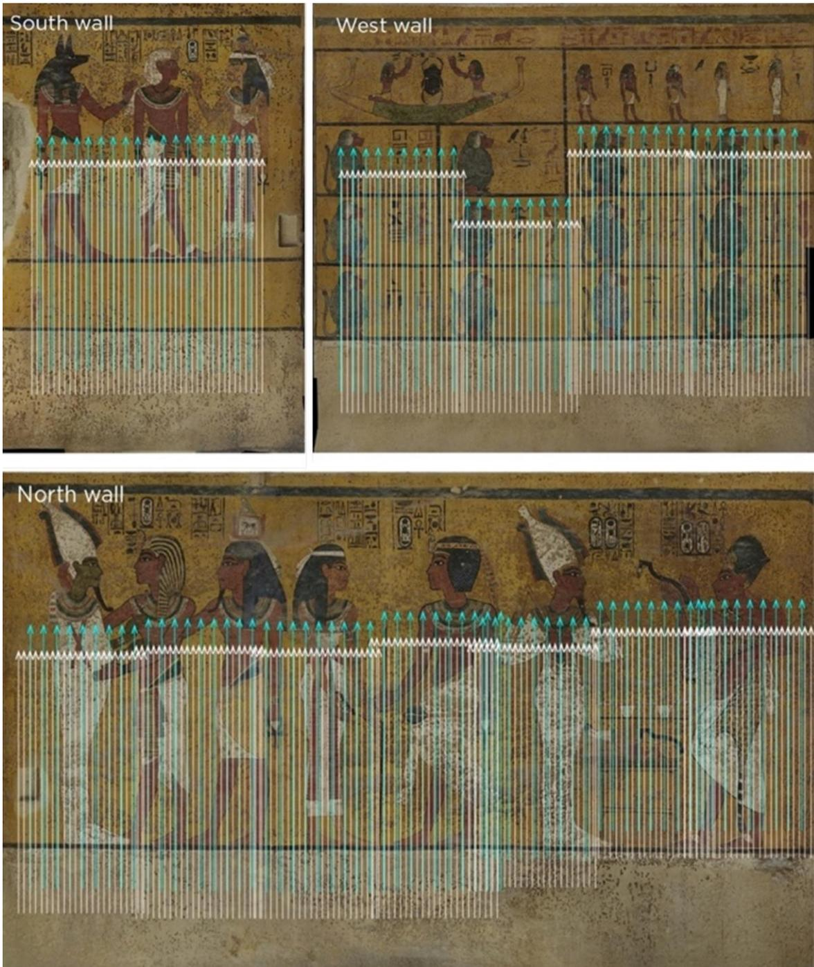
**Figure 3S:** IF radar profiles acquired with the multi-channel IDS Stream-C system along the KV62 walls, white arrows represent the position of the radargrams acquired in TM-mode, at fixed spacing of 0.0435 m; cyan arrows represent radargrams acquired in TE-mode at fixed spacing of 0.099 m.
