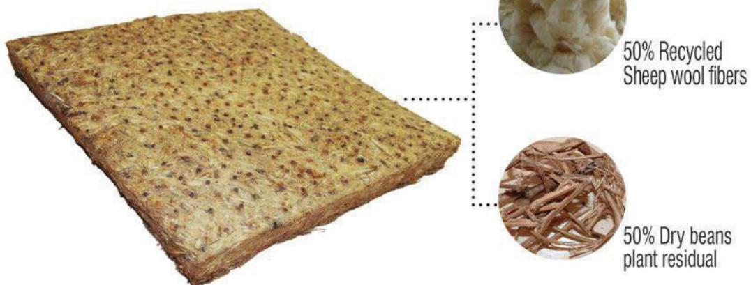
Figure 5. Sheep wool/Dry beans plant residual sample produced in laboratory composition.
