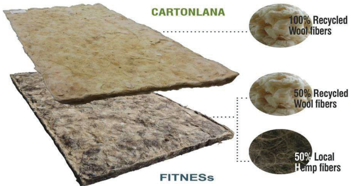
Figure 2. Cartonlana and FITNESs panels composition
