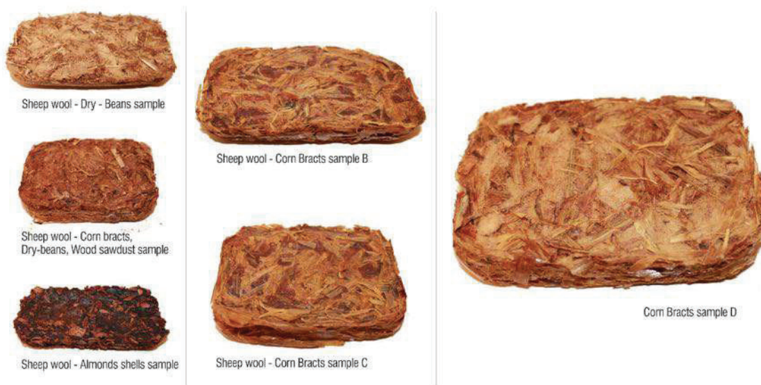
Figure 4. Samples produced in laboratory, combining sheep wool with different selected agri-food by products.
