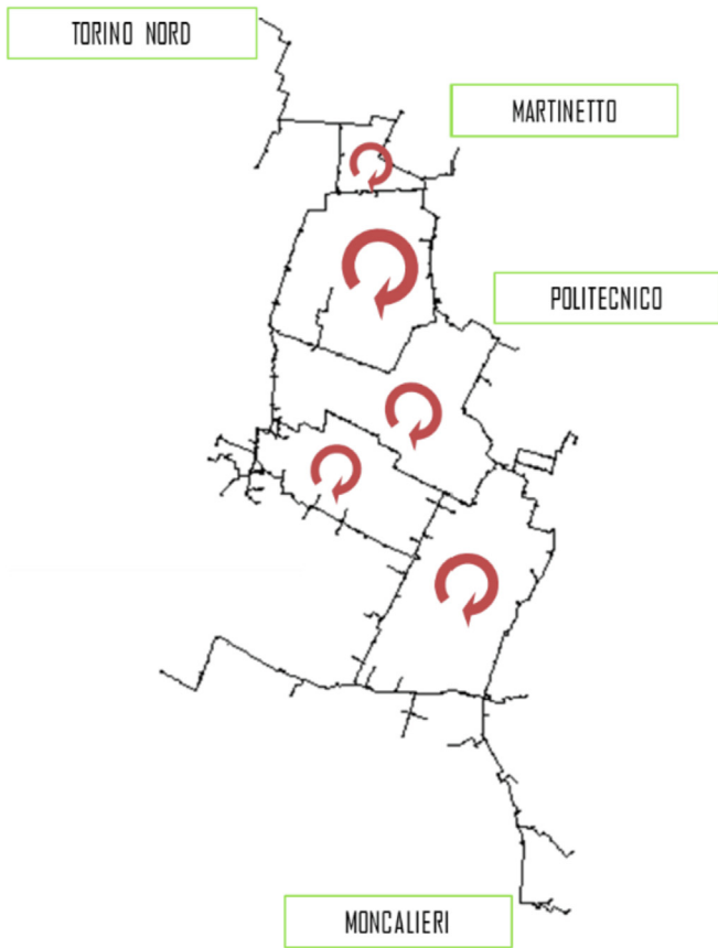
Fig. 4. Schematic of Turin transport line. In red the main loops.
