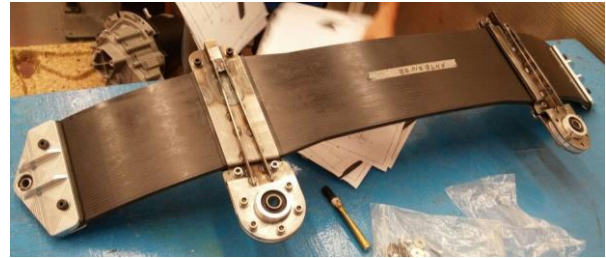
Figure 4. Manufactured CFRP transverse leaf spring
