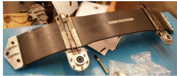
Figure 4. Manufactured CFRP transverse leaf spring
