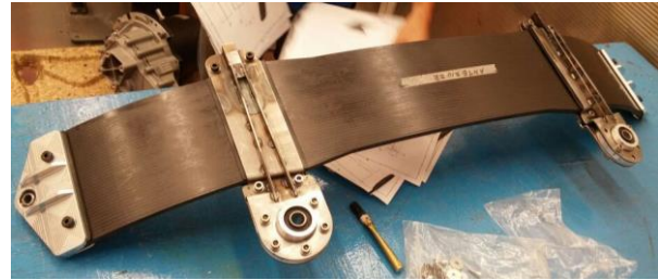
Figure 4. Manufactured CFRP transverse leaf spring
