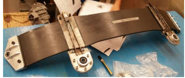
Figure 4. Manufactured CFRP transverse leaf spring
