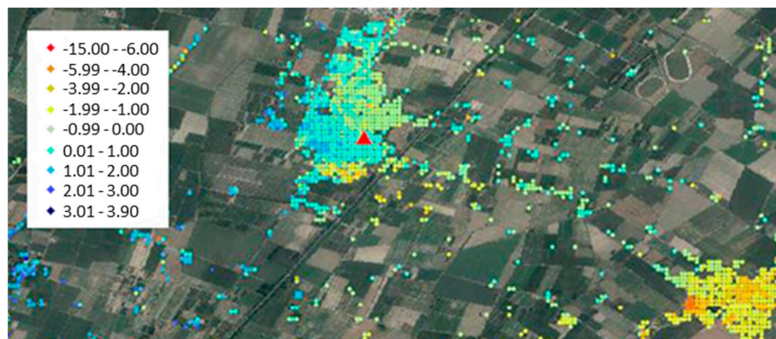
Figure 14. Example of vertical displacement velocities (mm/year) recorded from InSAR.
