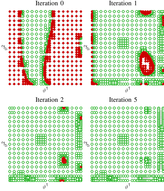
Fig. 9: Passivity characterization of the multiboard interconnect model illustrated after successive passivity enforcement (outer) iterations. Empty green (filled red) dots highlight passive (non-passive) parameter values for which no (some) SHH eigenvalues are detected by the proposed adaptive sampling algorithm.
