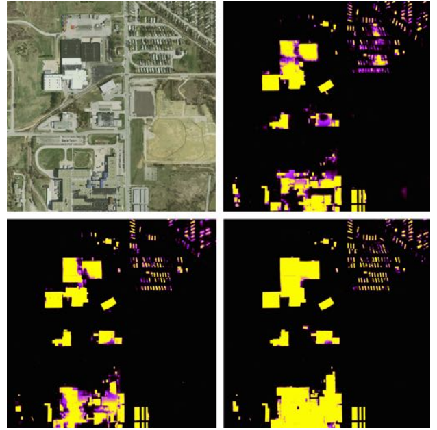
Fig. 4: Results over test area 6 in Bloomington city of INRIA dataset. The RGB input image is on the left. Score maps (Decoder SoftMax outputs) for the proposed network with 50, 101 and 152 layers follow. As the encoder depth increases, the quality of the score maps improves.
