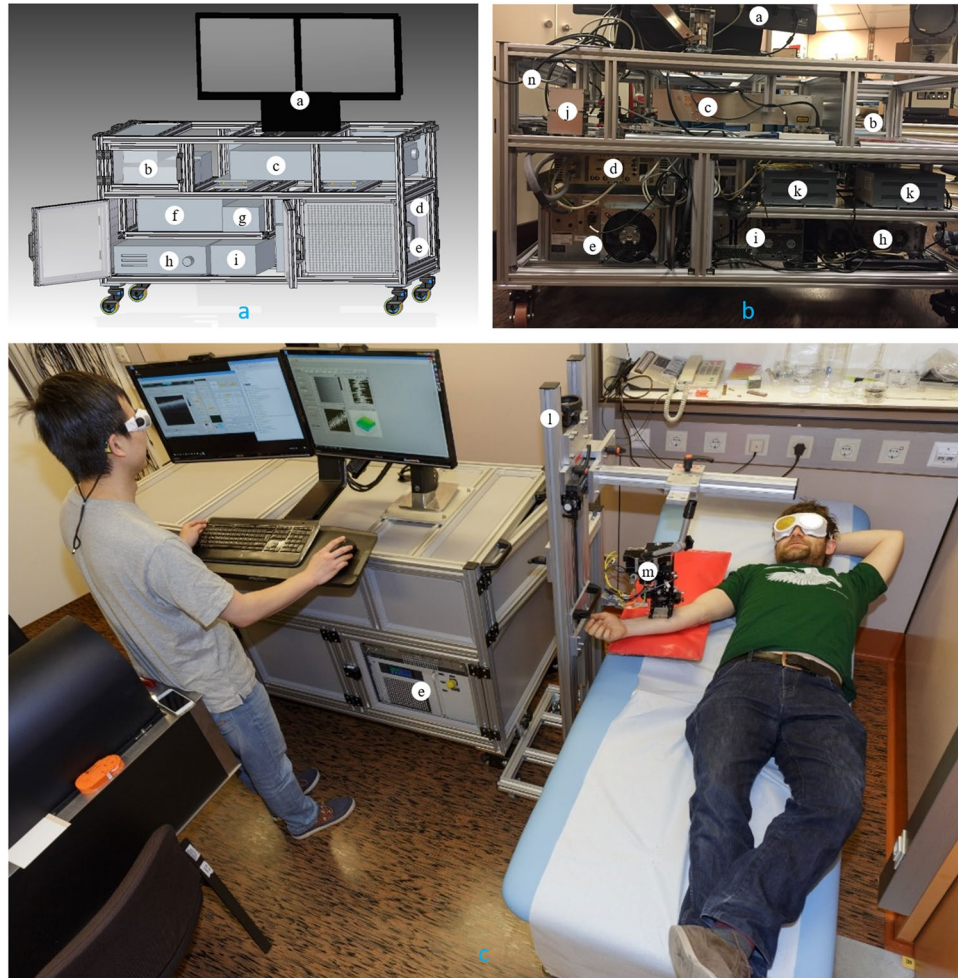
Figure 2. (a) Design of the cart. (b) Photo of the back side of the cart during assembling. (c) Illustration of the system during imaging. (a) Dual monitors; (b) storage compartment; (c) excitation laser head; (d) power supply and control unit of the excitation laser; (e) chiller of the excitation laser; (f) breadboard for OCT optics; (g) swept source; (h) PAT interrogation laser; (i) workstation; (j) servo boards for scanning mirrors; (k) power supply for servo boards; (l) rollable rack with an articulated arm; m: OCT/OCTA/PAT probe; n: compartment for probe storage.
