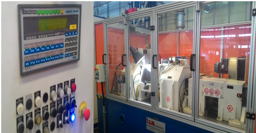
Fig. 3.7 The PLC interface and the ready to start test rig machine.
