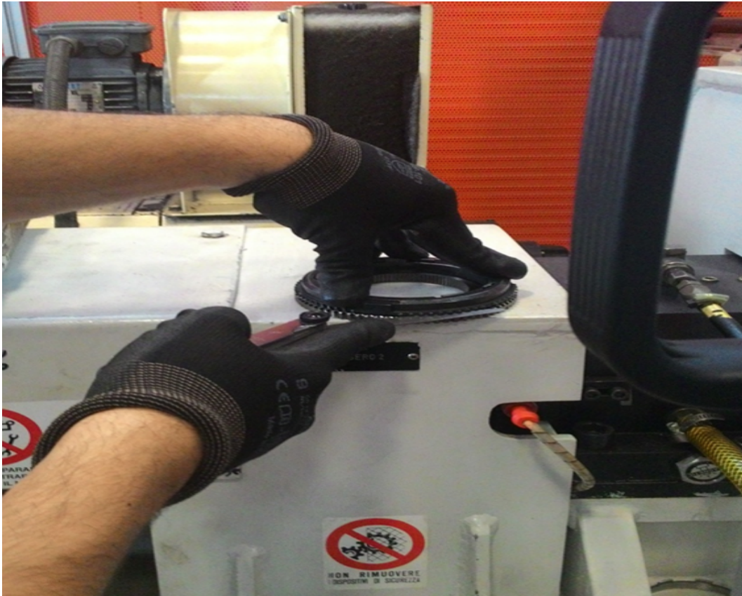
Fig. 3.6 Measuring the gap between synchro ring and clutch cone the synchro by feeler gauge.
