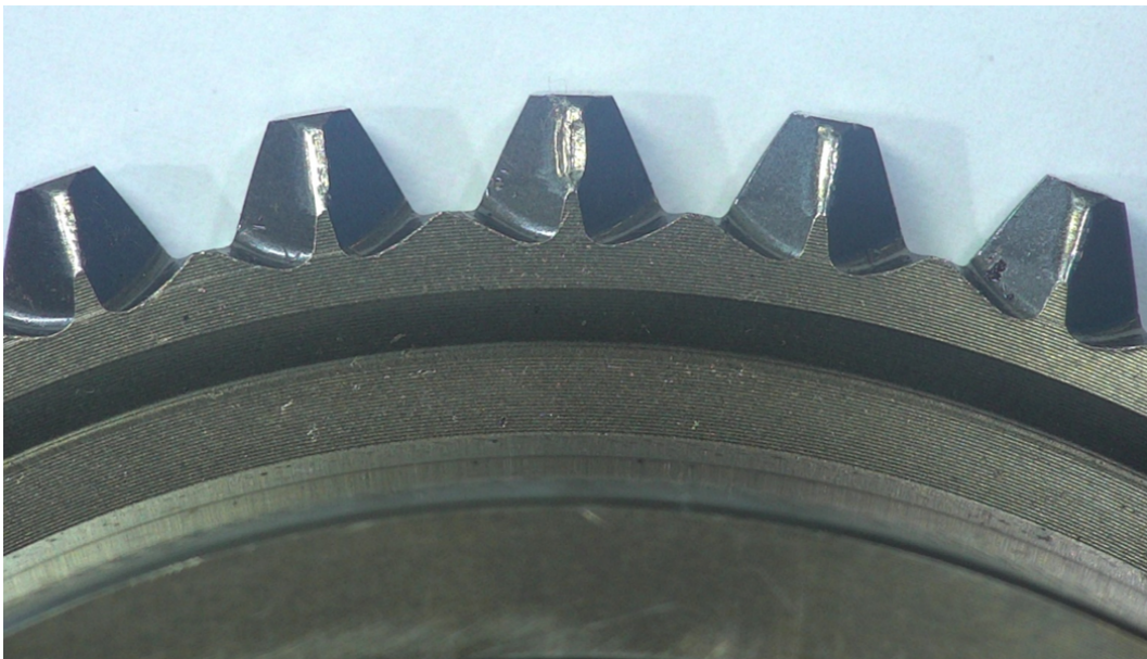
Fig. 2.14 An example of scraping on the gear teeth.
