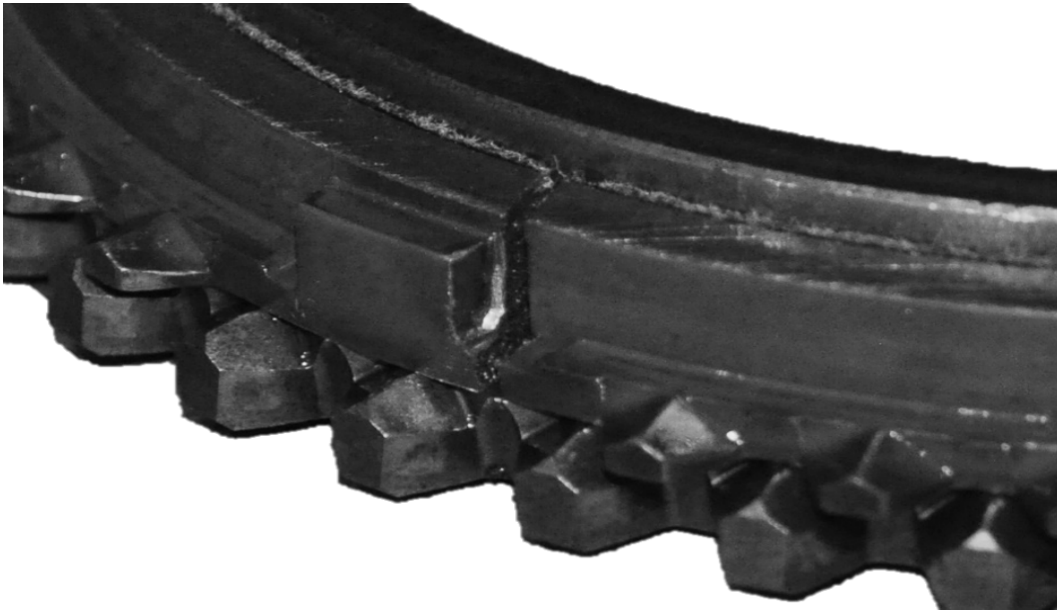
Fig. 2.15 An example of fracture area on the synchronizer ring teeth.
