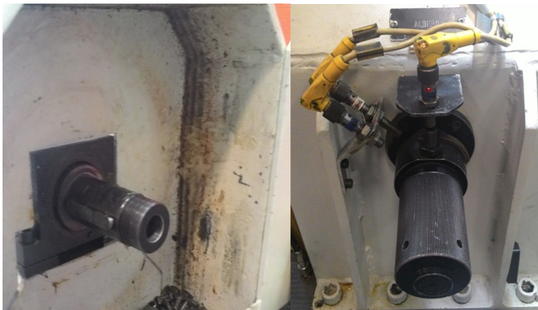
Fig. 3.3 The location of the inertia weight (left) and the sensor position (right).
