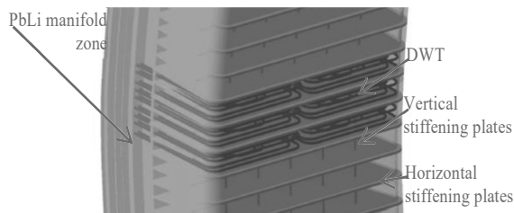
Fig. 2. WCLL 2018 OB segment: BZ and stiffening plates.
