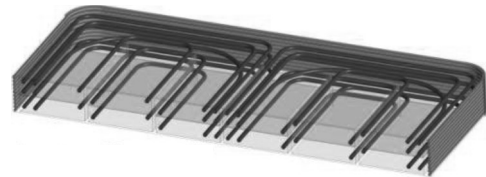
Fig. 3. WCLL 2018 OB equatorial breeding cell geometry.
