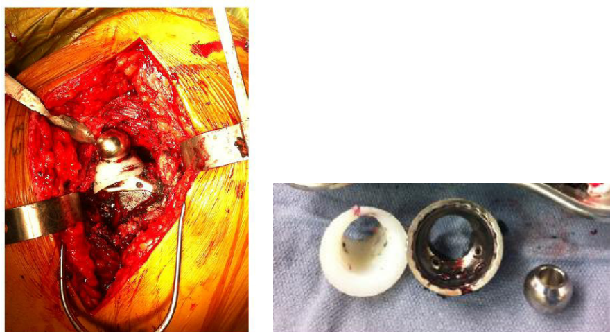
Figure 1.5 Photographs of the completed worn polymeric insert and metal cup by the metal head [10]
