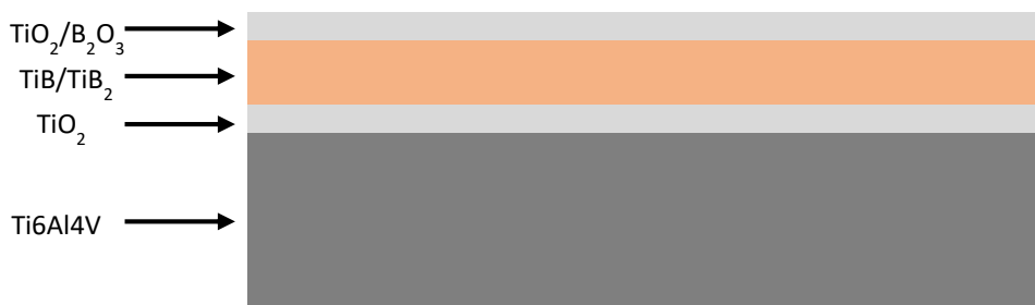
Figure 5.147 Scheme of the titanium borided coating for the samples without any pre/post treatment
