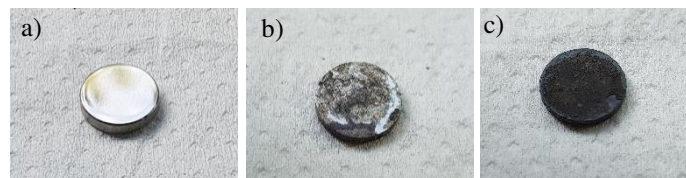
Figure 5.154 Picture of a) untreated sample, b) sample treated at 800°C for 3.5h and c) samples treated at 700°C for 3.5h
