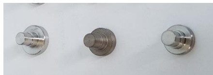
Figure 4.12 a) AISI 316L, b) treated Ti6Al4V alloy without any pre/post treatment and c) untreated Ti6Al4V alloy pins for fretting test
