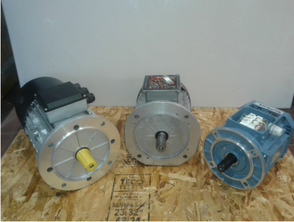
Figure 3.21: Picture of three tested SyR motors. From left to right: SR4kW, SR2kW2 and SR1kW1.
