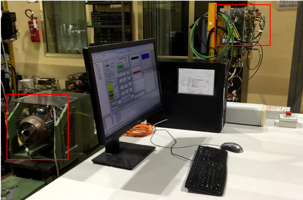
Figure 4.23: Experimental test bench for sensorless control of SyRM. Highlighted in red rectangles: motor under test and power electronic converter.
