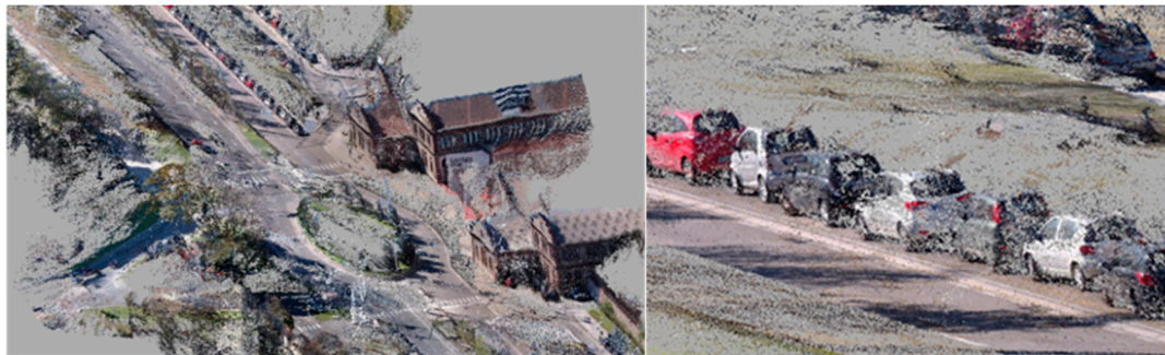
Figure 5. The resulting geo-referenced dense point cloud of the road infrastructure (on the right) and the detail of the parked cars.
